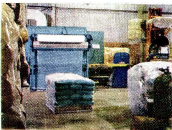
The packaging machine that wraps and seals an entire pallet of sacked monolithics in a tough polythene bag.
