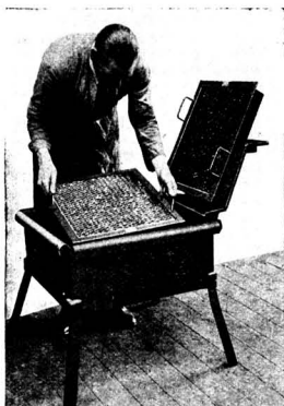
Fig. 6.—The Operation of Cleaning the Cells. (a similar Tank is used for Re-charging the Cells with Oil. Note the Shelf provided for Draining Purposes)
