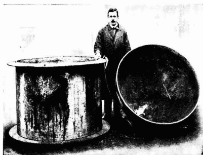
One of a pair of Aluminium Pans, 4ft. diam. x 6ft. deep, which failed around the centre seams and on the outlet pipes.
