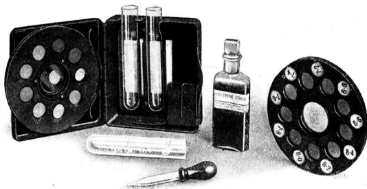
Lovibond Comparator showing Test Tubes and Standard Colour Glasses
