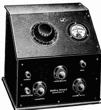
Fig 5. Dr. G. B. Harrison's Apparatus for pH Determination with the Glass Electrode
