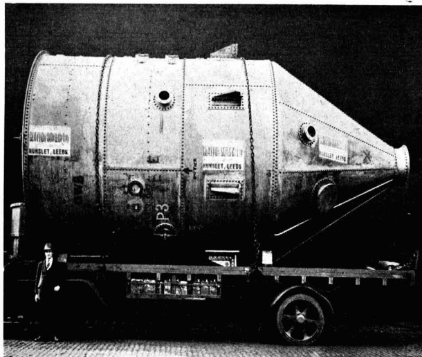
One of 13 vessels in STAINLESS STEEL, 13' 6" diam. recently made for IMPERIAL CHEMICAL INDUSTRIES.
