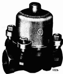
The Drayton Standard Industrial Steam Trap (balanced pressure) is suitable for all pressures of saturated steam from vacuum up to 120 lb. per sq. in. It has a very noticeable instantaneous action.
