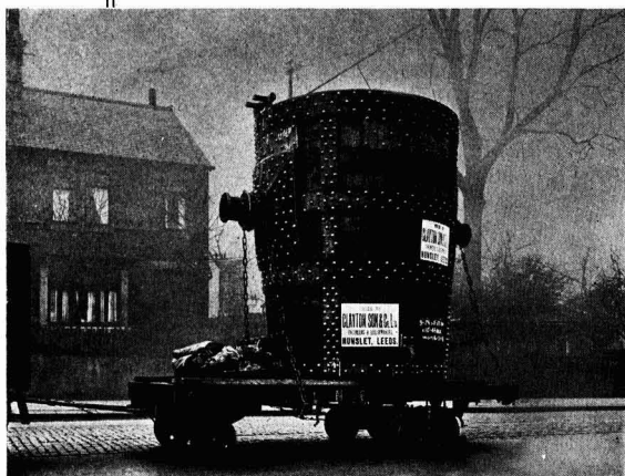
Mild Steel Ladle 9' 7 5 / 8 " × 8' 2 1 / 2 " diam. × 10' 4 1 / 2 " deep One of an order for four, for a British Steelworks.
