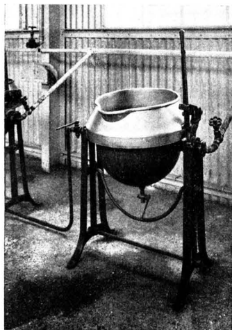
This small Monel metal kettle is one of a battery in use at the Lady Dane Cannery, Faversham, Kent.
