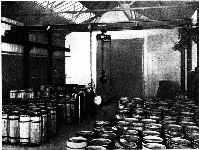
Above: These barrels of zinc oxide are neatly placed in the works store by the aid of a Morris Crane, the initial cost of which is very small.
