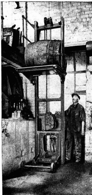
Above: The ingredients for "Walpamur" paint products are raised to the top of the mixing vessels by means of a Morris Stocker.
