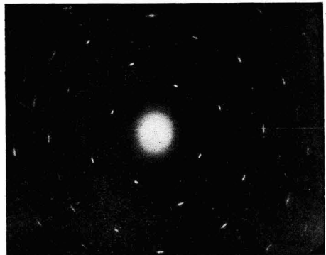
Electron Diffraction Transmission Pattern of an Aluminium Single Crystal.
