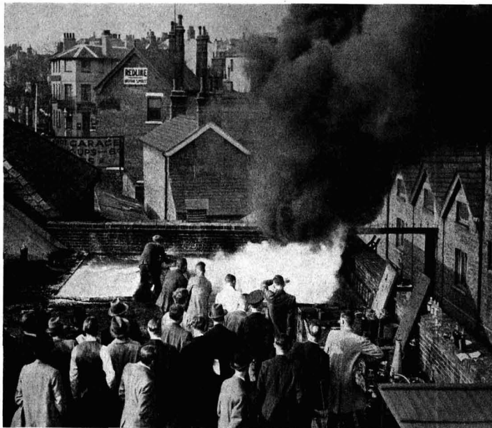
Extinguishing a blaze of 20 gallons of Fuel Oil at the demonstration at Richmond on March 28 by means of "Essex" Methyl Bromide Extinguishers
