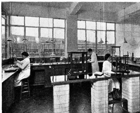
Standardisation Laboratory, showing special brick supports for Balance Bench.
