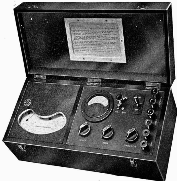
Millisecond Meter Test Set for the accurate measurement of very short time intervals on a direct reading scale.
