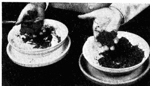
Monsanto Chemists showing what happens when equal amounts of water are worked into ordinary clay soil (left) and Krilium treated soil (right)
