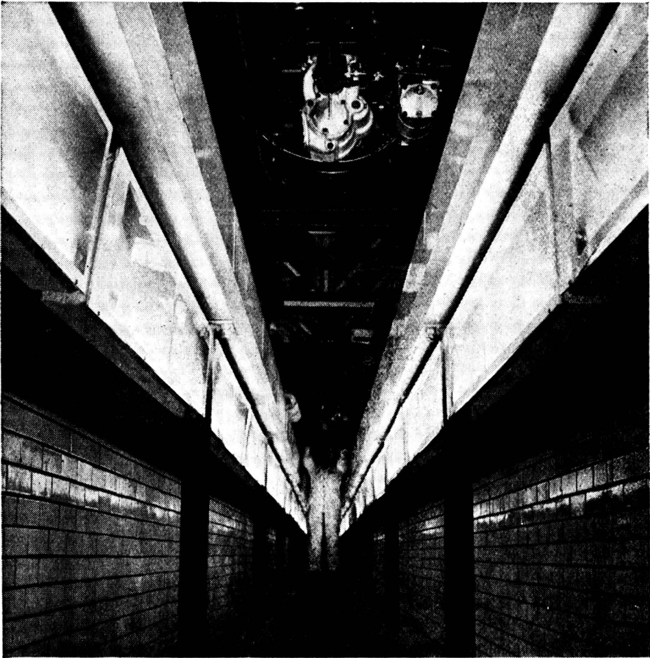
Pit beneath motor car assembly line for under-chassis work
