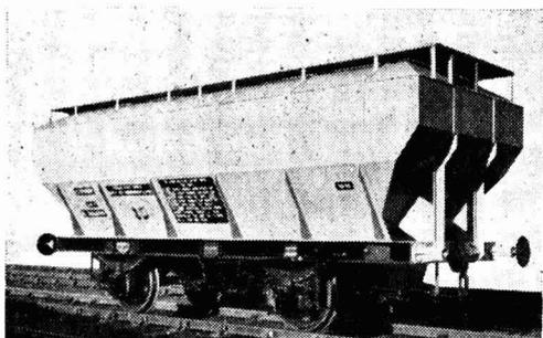
*A 24-ton covered hopper van for the conveyance of bulk chemicals*
