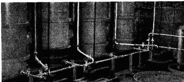
Purity of product is assured, because the clean homogeneous surface of the Glass permits of visual inspection at all stages. Ease of cleaning enables the plant to be changed rapidly from product to product.
