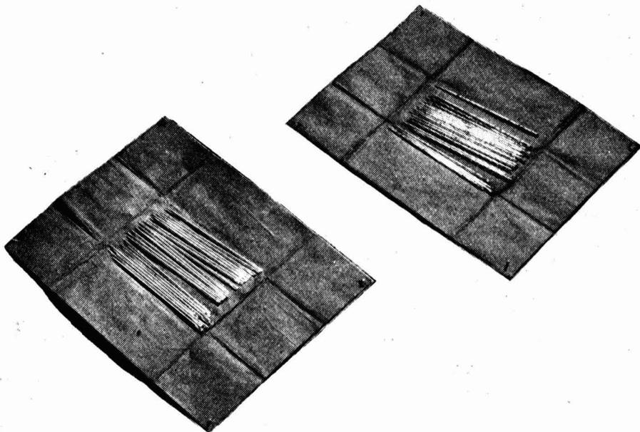
*Right: Nickel plated steel needles wrapped in 'purple' paper, showing heavy corrosion after a period of storage.
