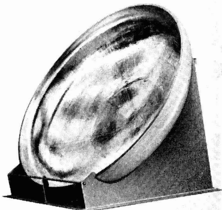
A 12 ft. 6 in. spun end in 'Colclad,' spun by Messrs. G. A. Harvey & Co., from a blank supplied by Colvilles, Ltd.
