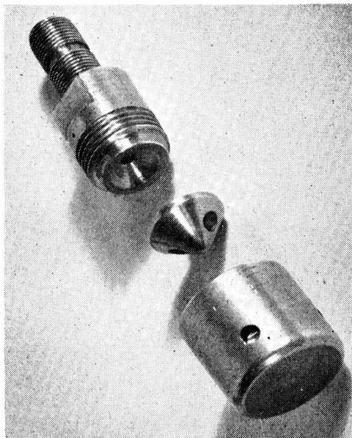
Fig. 4. Exploded view of cone-ring holder
