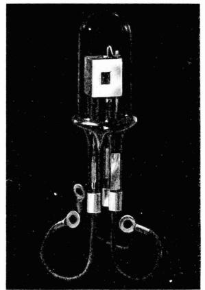
Vitreosil Hydrogen Discharge Lamps provide a source of continuous ultra-violet radiation for use in spectrometric investigations, including all types of ultra-violet absorption and hydrocarbon analysis, quantitative clinical measurements, medical and biochemical research.
