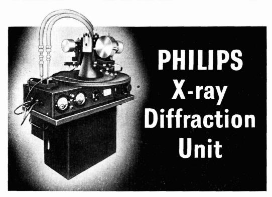
THIS apparatus constitutes the ideal flexible diffraction machine. With a power unit rated at 60 kvp. 20 ma. any of the modern technique can be readily employed. Among the many applications for this machine:—
