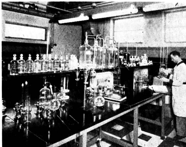
Part of the control laboratory. The assistant is performing an electrometric titration
