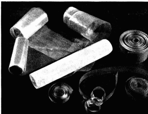
**'Fluon' tape as used in the chemical and electrical industries; the tape is cut from a block as shown opposite**
