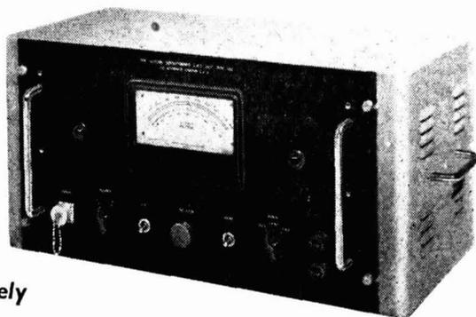
**from stock.** This standard Isotope unit, designed for nucleonics but suitable for many electronic requirements has **EXTREME STABILITY** (0.05% for 10% change in mains input voltage), **HIGH CURRENT OUTPUT** (3 mA), E.H.T. FROM 300 - 3000 VOLTS (negative and positive polarity).
