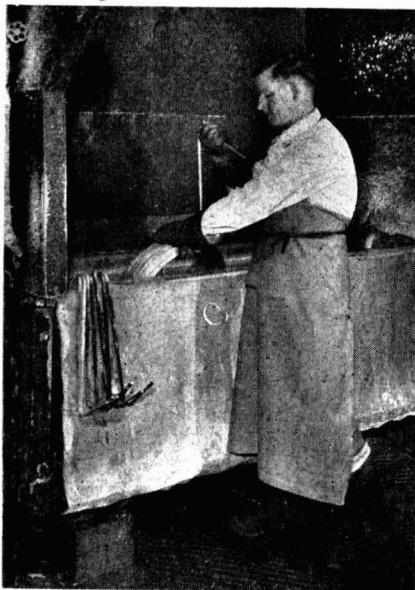
Wearing 'Terylene' overalls, an I.C.I. Metals Division worker cleans metal strip in an acid bath
