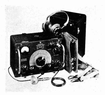
Complete kit for the Dawe ultrasonic thickness gauge Type 1101B
