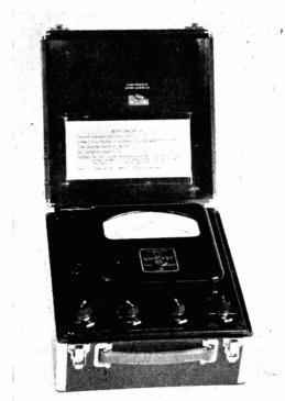
Cambridge corrosion voltmeter, readily transportable
