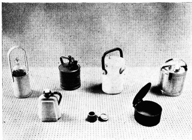
Handling aids for dangerous liquids: A Winchester carrier, a container with a safety spring cap, a stainless steel container for nitric acid with a screw cap, unbreakable polythene containers, a heavy container for bench use and a container with the lid held open by a celluloid link. If the material in the latter catches fire the link is destroyed and the lid drops
