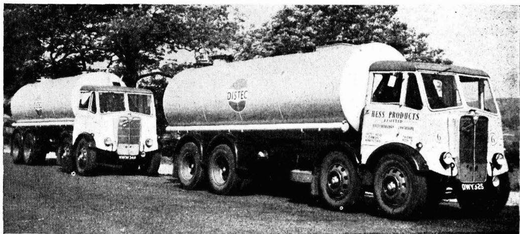
Two tankers now used regularly for road despatch of bulk quantities of Distec fatty acids. They are stainless steel of the single-compartment type and have pumps and heating coils fitted. Each carries 12-tons of fatty acids. The Distec range is made in Hess Products' Fractional Distillation Unit at Littleborough, nr. Rochdale. In the near future they will also be making the Armour range of nitrogen derivatives of their fatty acids which will be offered for sale by Armour & Company Ltd., of London
