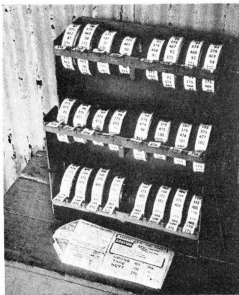
This dispenser carries gross tare and net weight labels in roll form to provide for a range of tare weights from 87-110 lb at 1 lb intervals
