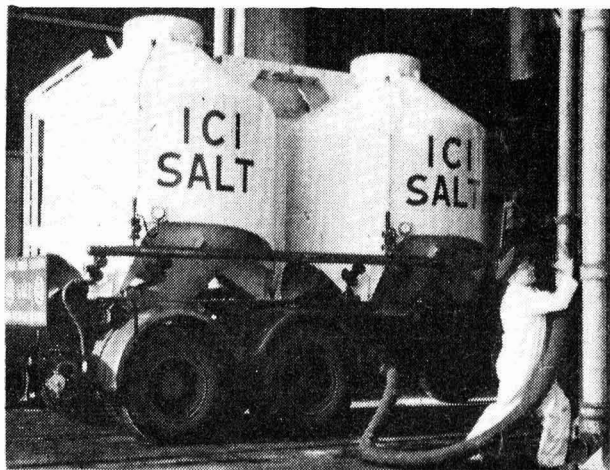
Bulk delivery of pure dried vacuum salt is performed by this special vehicle introduced by ICI Salt Division. Salt is pumped by compressed air direct from the vehicle to the customer's premises
