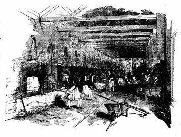
BELOW: The illustration concerns manufacture of soap in 1840. It shows how oils or fats were boiled with caustic soda in deep open-top buts, or pans, known as 'kettles,' to form soap and glycerine. Hot oil or molten fat is being
