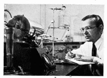
Two typical views of BF Goodrich research workers in action are shown on this page. The researcher on the left is conducting microanalysis for carbon and hydrogen to determine the chemical composition of a research sample
