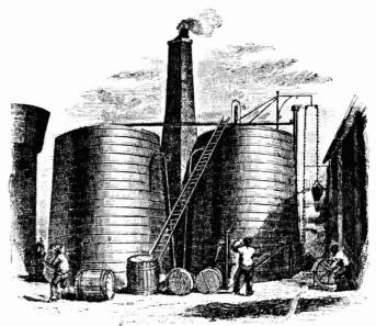
RIGHT: Another view at the works of Kurtz, Cropper & Co., of Liverpool (1844), showing the sublimers and drying furnaces used to get rid of the impurities that existed ammonium chloride after its first crystallization. Regulation of heat was an important factor in this process
