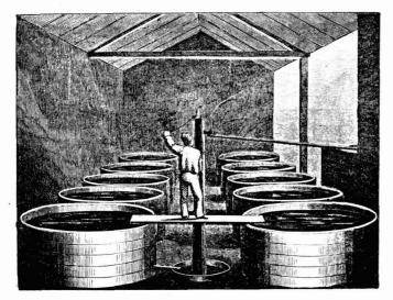
LEFT: Here are shown tubs used in 1844 for crystallizing ammonium chloride. A contemporary account of the process states that the salt crystallized out in four to six days, according to the state of the weather. Note the precarious position which the workman occupies. Would the present day factory inspectors allow this?
