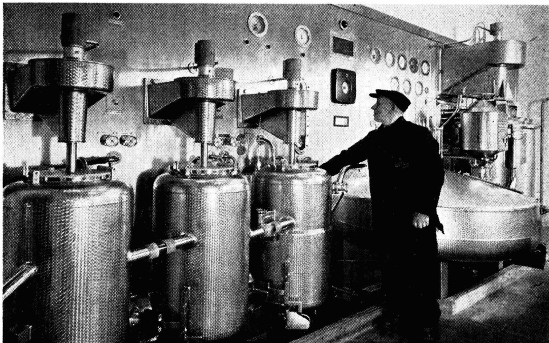
Biazzi plant at Ardeer. In line are three washing vessels connected with the separator. Beyond is the nitrator. Mr. William Boyd is the 'operator'
