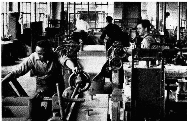
The millroom showing triple roller mills. A film of paint is running from the mill in the centre of the room
