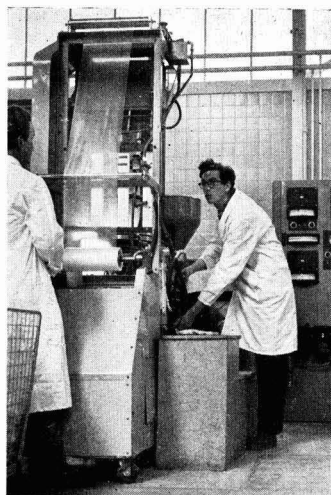
Left, architect's impression of the entrance to the laboratories. Above, an experimental Alkathene being extruded to determine its processing qualities and the properties of the film made. A major aspect of the work of the department is that of developing new and improved materials and conversion techniques. Below, layout of the departments at the research and development laboratories
