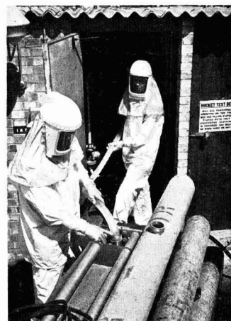
Protective suits in use on the rocket test beds of the de Havilland Aircraft Co.
