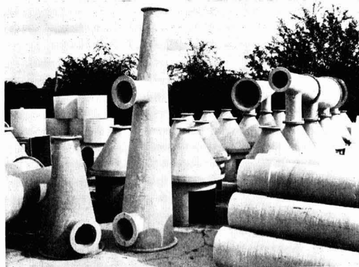
Ducting, cowls and stacks for a fume extraction system at a preserve factory made from Bakelite polyester and epoxide resins reinforced with glass fibre material by Mendip (Chemical Engineering) Ltd.
