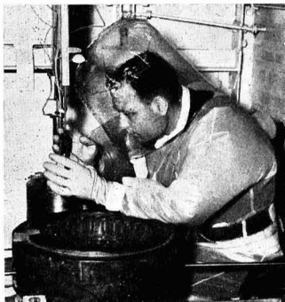
Safety foreman, Mr. Leslie Jones, wearing a pressurised protective outfit, inspects apparatus in a highly active analytical cell. Operations in this cell are remote controlled
