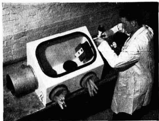
The Mark III glove box made by H. and E. Lintott Ltd. which has an air filter and ejector and alternative methods of transfer through a posting bung or an internally removed bung
