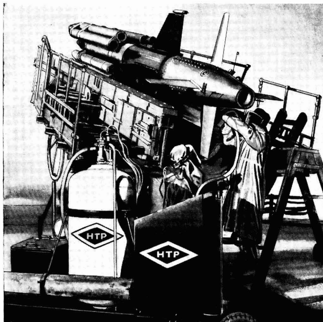
A missile being fuelled with high test peroxide
