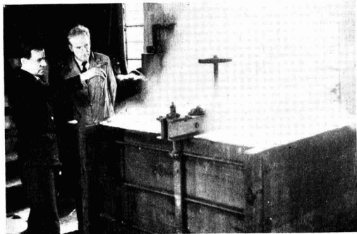
NIFES engineer points out to a dye-house manager the considerable wastage of steam from the unenclosed dye vat
