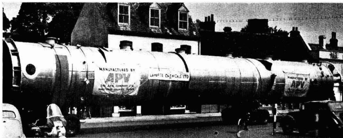
This aluminium extraction column, 80 ft. long by 9 ft. diameter, is one of six being made by the APV Co. Ltd., Manor Royal, Crawley, Sussex, for Laporte Chemicals Ltd. for the production of hydrogen peroxide. Its fabrication involves the welding of aluminium up to 1½ in. thick. Shown passing through Dunstable, Beds, the column is claimed to be one of the longest objects to travel by road, the overall length of the vehicle and column being 104 ft. It left APV's Crawley works on 30 May and reached Warrington on 3 June
