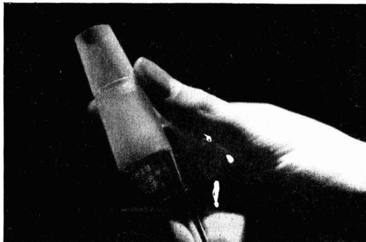
P.t.f.e. sleeves made by Loughborough Glass Co. These are fitted to ground glass joints to prevent sticking and are claimed to replace greasing
