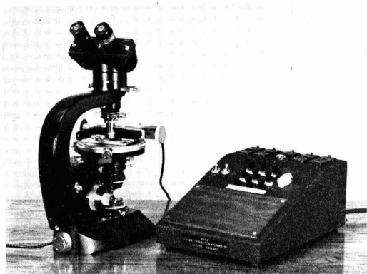
Point counter by Cooke, Troughton and Simms Ltd. which can be used for particle counting or blood cell analysis
