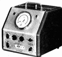
Master pH meter made by W. G. Pye and Co. Designed as a direct reading instrument it works in the two ranges 0-10 and 4-14 pH
