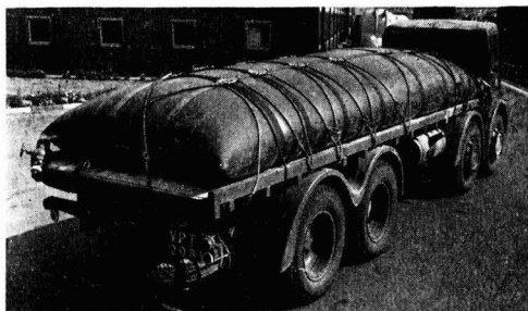
Portolite flexible container, with 2,000 gall. of I.C.I. iso-octanol, starts its journey from Billingham
