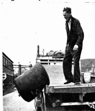
Testing corrosion-resistant 50 gall. drum by dropping it from a lorry. These drums are made by Fireproof Tanks Ltd. from rayon, coated and impregnated with British Geon's Hycar nitrile rubber. They can easily be folded when not in use. Owing to an error in transmission, this drum was incorrectly illustrated in 'Chemical Age,' 27 August, p. 323
