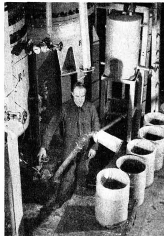
Bowater drums with loose plastics liners being filled with alkyl synthetic resin in the polymer emulsion plant of Scott Bader and Co. Ltd.
