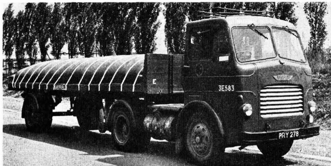
British Road Services have approved Dunlop collapsible containers and seen here is a 24 ft. semi-trailer with 2,000 gall. of liquid
