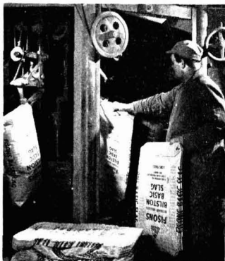
A Bowater multiwall paper sack is placed on the filling spout for a load of Bilston basic slag at one of Fisons' plants
