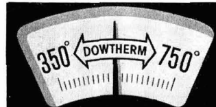
Process Heating. Dowtherm* A—heat-transfer medium provides precise temperature control at low pressure for process heating in the 350-750 F. range.
