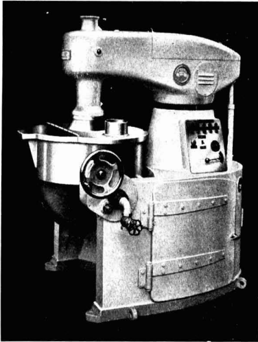
Heavy Duty Hydraulic Mixing Machine for caramel, nougat, etc., 1½ to 3 cwts. capacity, Type 16 PD.
