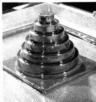
Vacuum forming possibilities in Makrolon illustrated by R. H. Cole
