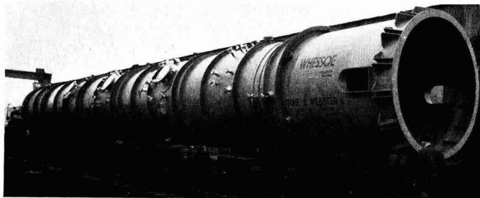
Whesoe Limited have recently delivered this 115 ft. high large-diameter high vacuum fractionating column, weighing over 60 tons, to Shell's refinery at Stanlow. The column will be part of the new paraffin and microcrystalline wax plant which is now under construction at the refinery by Stone and Webster Engineering Limited
