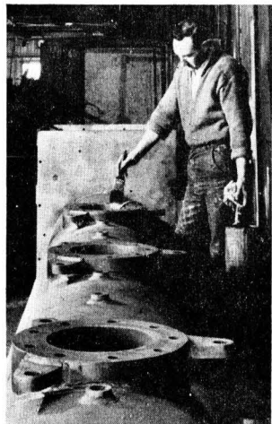
On large metal structures, such as this air duct of A. Reyrolle and Co. Ltd., Kephos is simple to apply by brush
