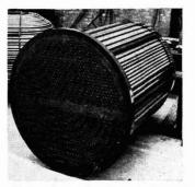
Heat exchanger bundle, part of a unit produced by William H. Capper for D.C.L.
