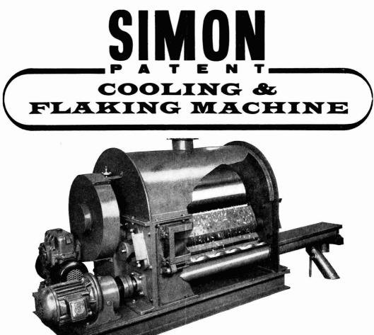
In constant production in a large number of sizes ranging from 8'' dia. x 8'' long to 42'' dia. x 108'' long. Rolls are constructed of cast iron, chromed cast iron, nickel iron, stainless steel, phosphor bronze, etc.
