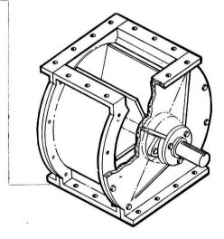
THE FULLER VANE-TYPE FEEDERS for handling pulverized and granular materials are employed wherever controlled flow and discharge of materials from bins, silos, etc., is required. They may be used as air locks for positive or negative pressure differentials and are available in capacity ranges to meet normal plant requirements and are built with circular or rectangular outlets.
