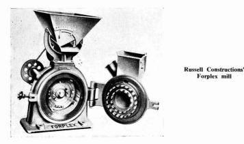
a rotating disc or rotor fitted with concentric hammers running between the teeth of a disc located on the floor of the mill chamber. The particles of material being ground are subjected to continuous and high frequency attrition between the high speed rotary and the static grinding element and are thrown by centrifugal force against a circular drum in the form of a screen or slotted plate which surrounds the periphery of clog the surrounding screen or slotted plate.
