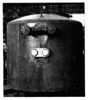
Pressure filter, 7 ft. 6 in. dia. and 7 ft. high, fabricated by R. White and Sons (Engineers) Ltd., Widnes, Lancs, who are shortly extending their fabricating department to accommodate larger vessels and offer quicker deliveries
