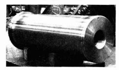
An example of the work of Hadfields Ltd., East Hecla Works, Sheffield 9, who are engaged in the manufacture of forged vessels for very high pressures, is this composite vessel for production of high pressure polythene (photo by courtesy,
