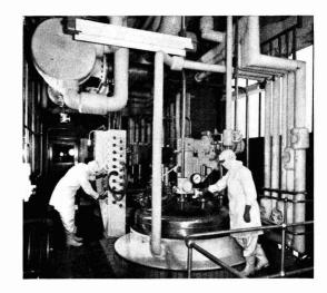
This view of two crystallisers in the new Distillers Co. (Biochemicals) Ltd. plant shows the use of a pipe connection panel. This system greatly simplifies pipe layouts and makes effective sterilisation possible
