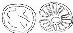
Fig. 1 (left): Print from drop of cuprammonium solution Fig. 2 (right): Print after addition of castor oil
