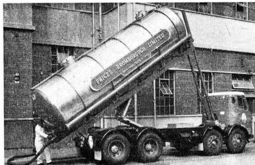
The new road tanker in the tilted position
