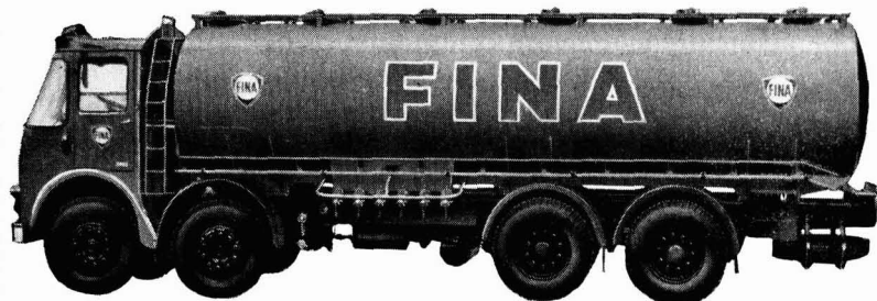
4,000 GALLON 6 COMPARTMENT MILD STEEL SPIRIT/OIL TANK, MOUNTED ON ATKINSON CHASSIS MODEL L. 1786, FITTED WITH VARLEY DH 100 PUMP.
