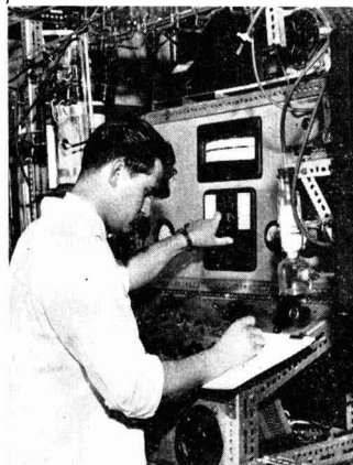
Dexion alloy slotted angle is used extensively in the research department of Simon-Carves Ltd., Stockport. Apparatus shown here is for the study of catalytic processes, including the detoxification of town's gas and the removal of sulphur compounds from fuel gases
