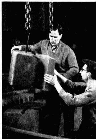
This 'shot' from the film 'Carbon dioxide for steel foundries' shows the placing in position of a section of the mould. Sections are assembled in sequence
